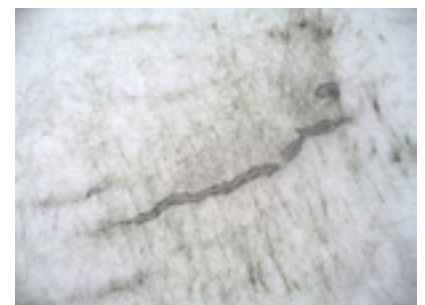
Image 3: Effect of stiffer surface due to thick lacquers. In some circumstances the lacquer substrate can generate deep cracks to the PVC coating.
