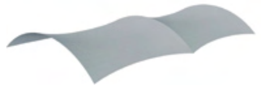
Figure 3: the arch supported or barrel form
